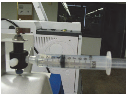
Figure 6.36. Removing the Methanol from the Sparge Vessel
