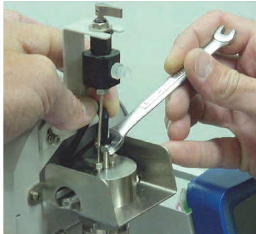
Figure 8.9. Tightening the Foam Buster heater/thermocouple nut
