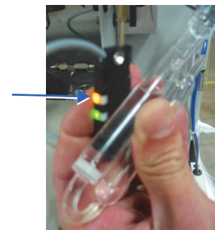
Figure 10.6. Liquid in the sparge vessel actuates the sensor
