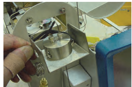
Figure 8.6. Installing the sparge mount bracket
