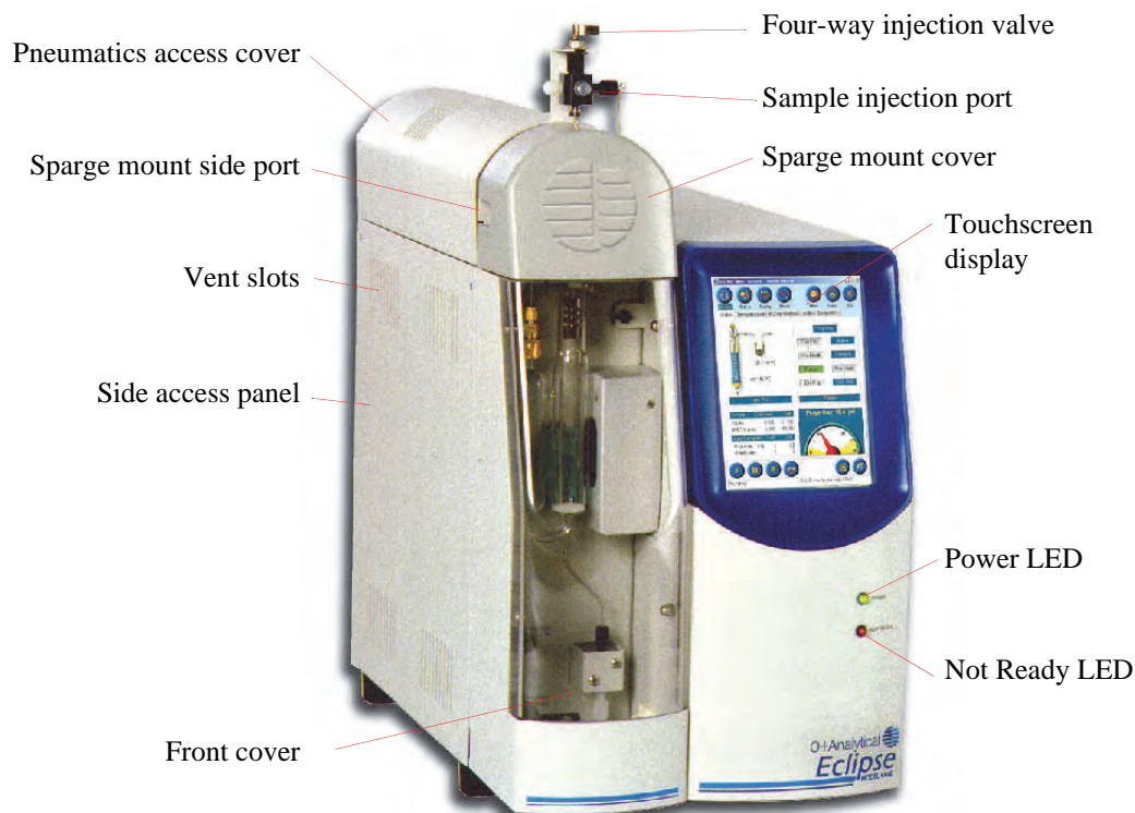
Figure 2.1. Eclipse front exterior components
